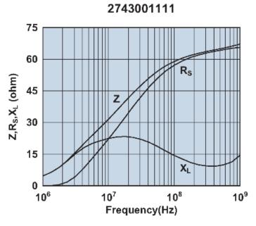
Impedance, reactance, and resistance vs. frequency.
