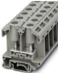
Universal terminal block with bolt connection, cross section: 0.1 - 25 mm 2 , width: 18 mm, color: gray
