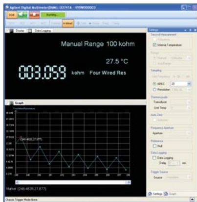
Figure 2. Example of the U2741A AMM Graphical User Interface
