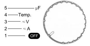
Figure 4. Rotary Switch
