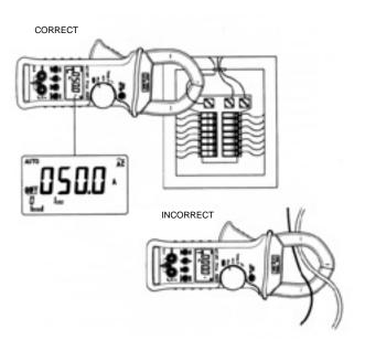
Figure 17. Measuring AC Current.
