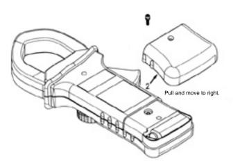
Figure 27. Step 2 of Battery Replacement.
