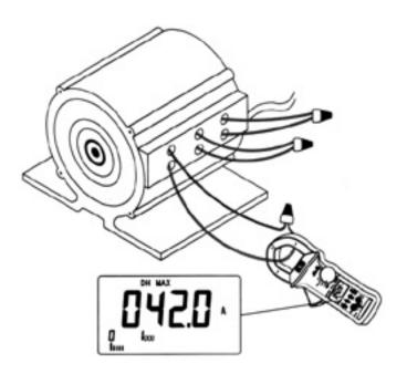
Figure 19. Measuring AC Motor Curent
