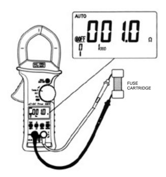
Figura 21. Measuring Resistance and Continuity.
