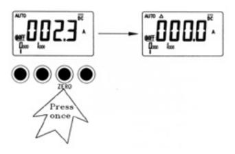
Figure 9. relative(Zero) Operation.
