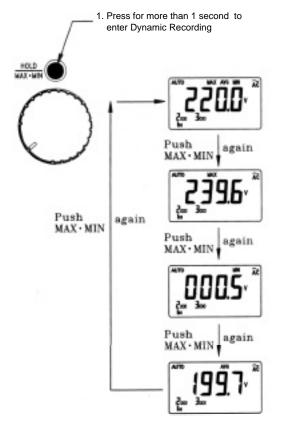
Figure 7. Display of Dynamic Recording
