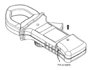
Figure 26. step 1 of Battery replacement.
