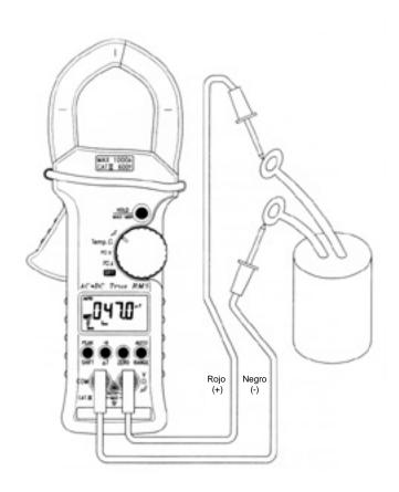
Figure 24. CAPACITANCEMEASUREMENTS.
