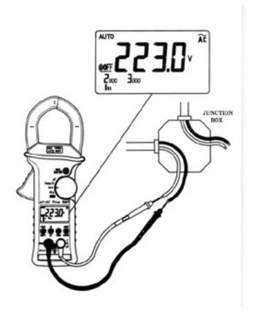
Figure 20. Measuring Voltage.
