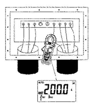
Figure 18. Measuring AC Curreft
