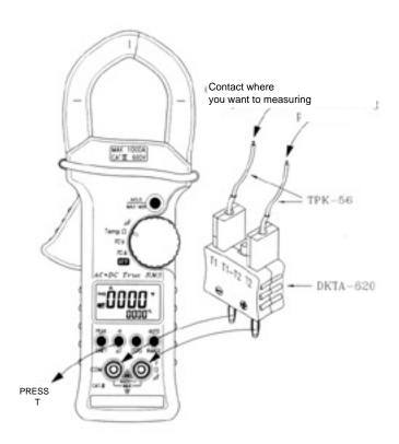
Figure 23. Measuring Temperature on Refrigeration System.
