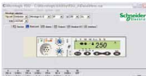
RSU mini-supervision screen for current measurements.
