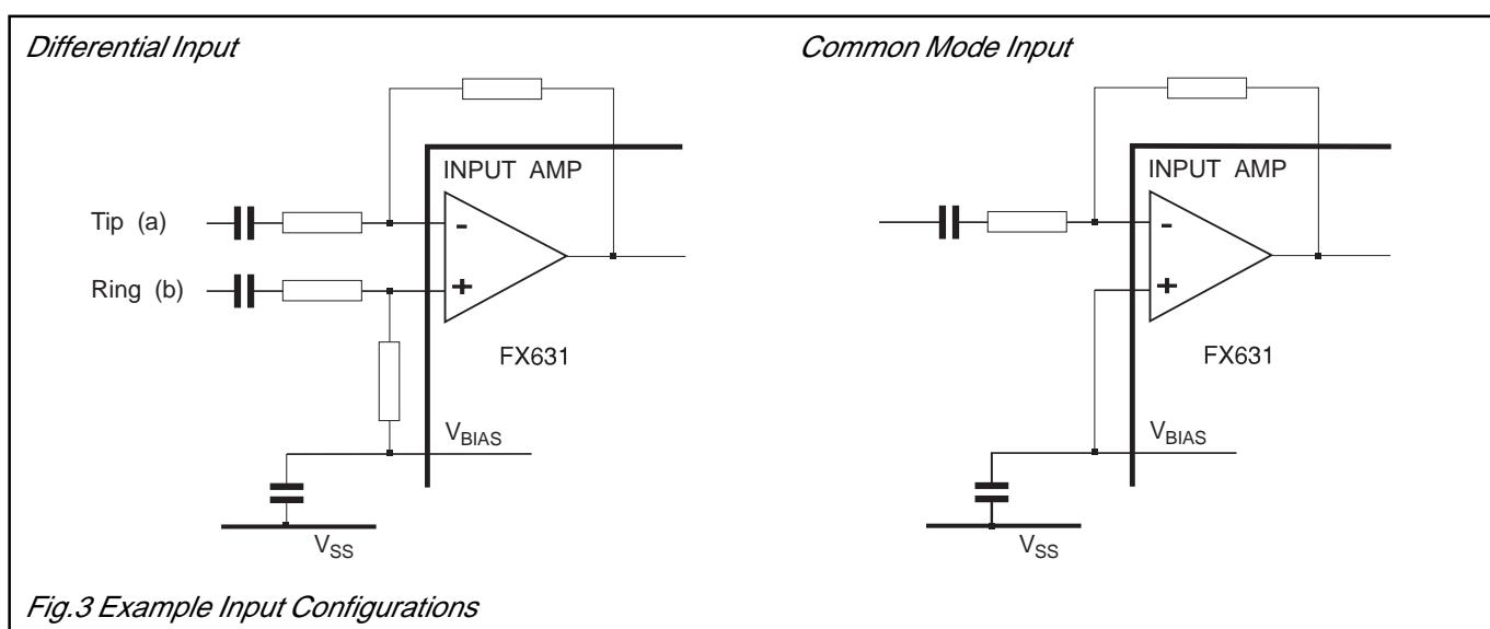
Fig.3 Example Input Configurations
