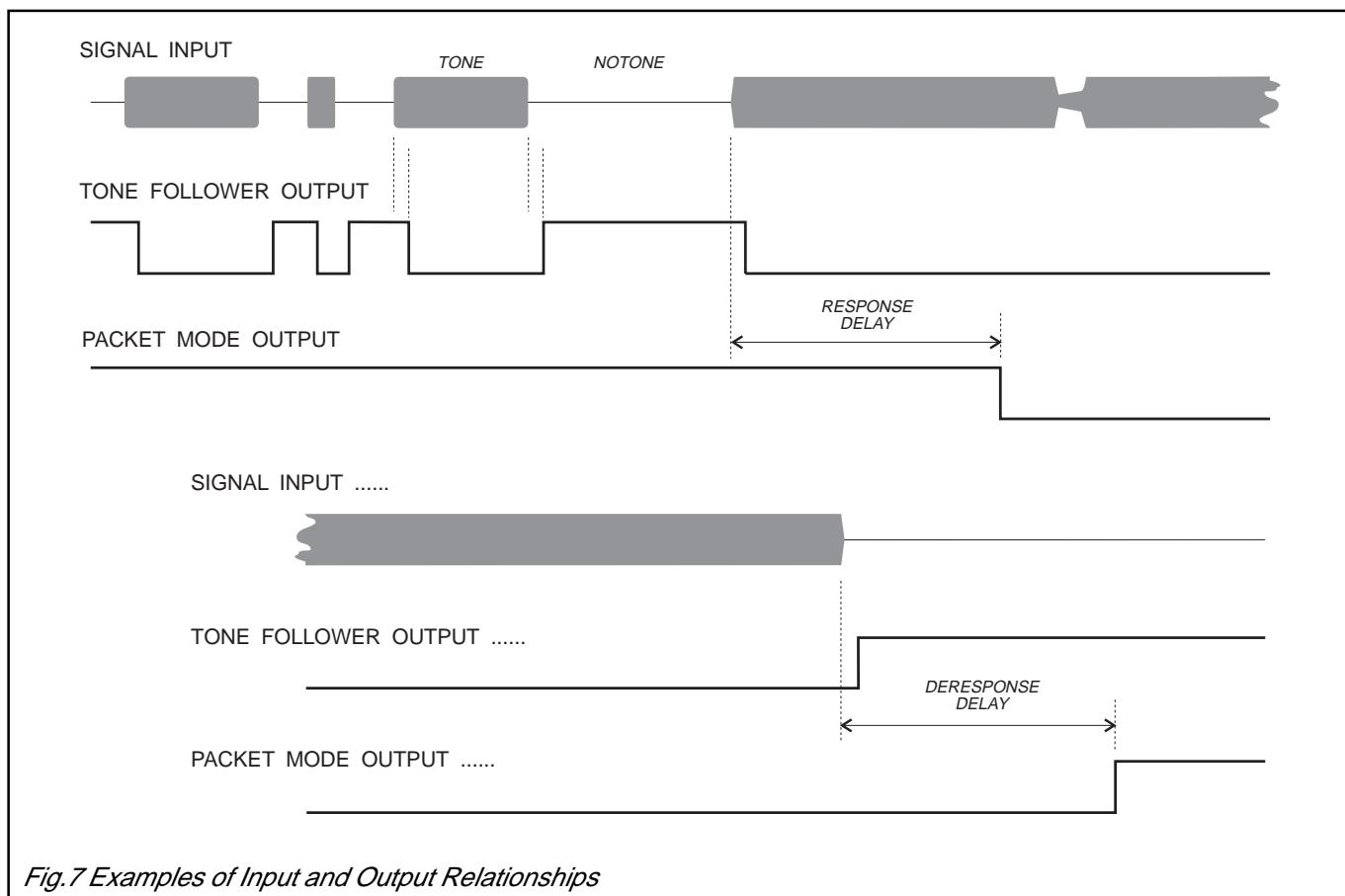
Fig.7 Examples of Input and Output Relationships
