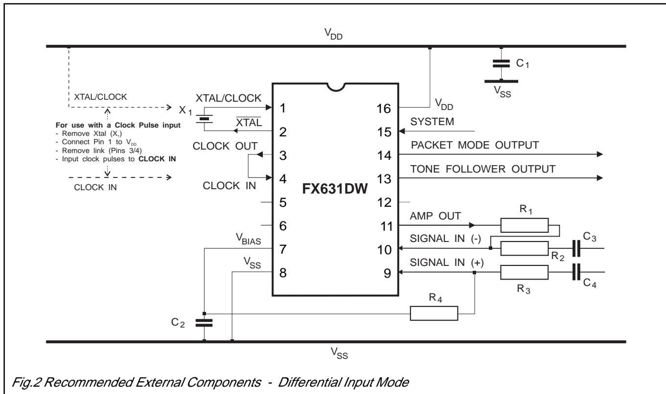
Fig.2 Recommended External Components - Differential Input Mode
