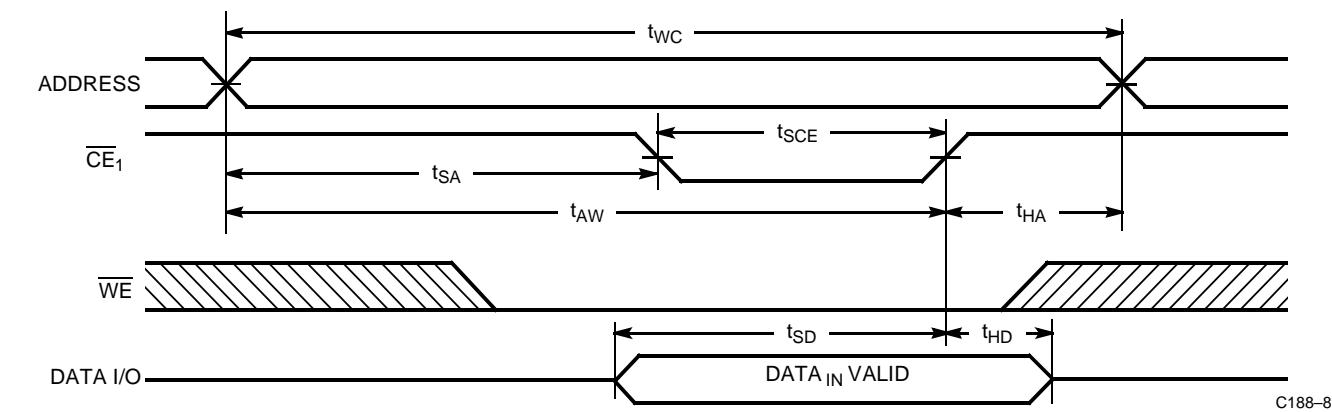
Write Cycle No. 3 ( $\overline{WE}$  Controlled,  $\overline{OE}$  LOW)<sup>[9,13,15]</sup>
