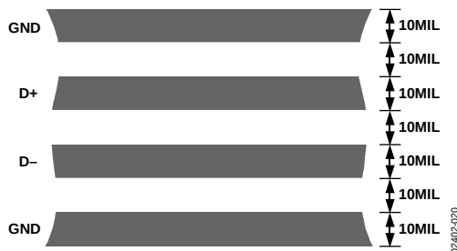
Figure 20. Arrangement of Signal Tracks
