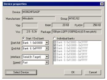
First carefully select the correct target device. A false selection may damage your target! Then select the chip area you would like to access, the sectors of the on chip-flash and the interface you would like to use. The parallel interface requires a parallel programming socket; the serial interface requires a cable to connect FLASHER to your target.
