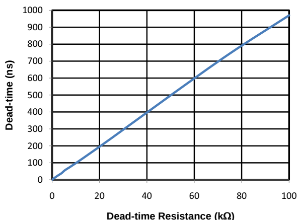
Figure 37. Dead Time vs. Resistance ( R_{DT} )
