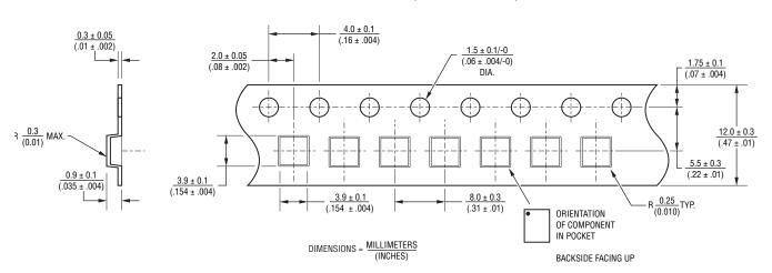
Devices are packed in accordance with EIA standard RS-481-A and specifications shown here.
