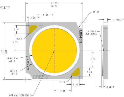
Tc measurement point: either the anode or cathode solder pad
