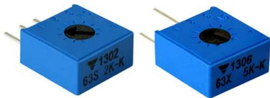
The Model 63 cermet trimmer is available in several pin configurations for top or side adjustment and with a choice of Knob styles for finger setting. Quick adjustment is achieved with multi-finger wiper and the standard resistance range is between 100  $\Omega$  and 2 M $\Omega$  with a tolerance of  $\pm 10\%$ .
