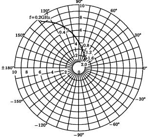
$\begin{array}{l} S_{12e} \\ V_{CE} = 5V \\ I_{C} = 5mA \\ Ta = 25^{\circ}C \end{array}$
