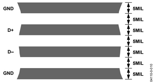
Figure 22. Typical Arrangement of Signal Tracks
