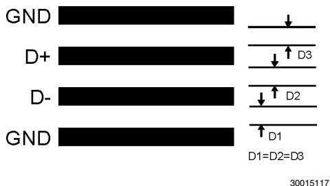
FIGURE 8. Ideal Diode Trace Layout
