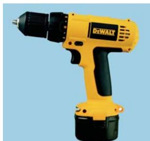
9.6V drill/driver suitable for drilling and screwdriving applications. Two speed settings, variable speed and reverse action for maximum control. Fourteen position adjustable torque control for consistent screwdriving in all materials. 10mm keyless chuck with automatic spindle lock for quick and easy bit change. Supplied with one hour charger, 2 x 1.3Ah Ni Cd battery packs and carry case.
