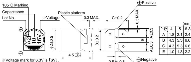
Type numbering system (Example : 16V 10 $\mu$ F)
