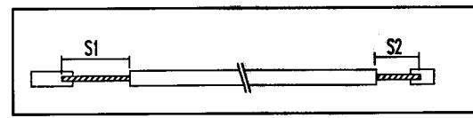
\* Note : The overlapping length of insulation on the conductor at the pre-stripped end is approximately 1 mm.
