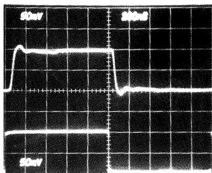
Top Trace: Output; 50mV/Div., 200ns/Div. Bottom Trace: Input; 50mV/Div., 200ns/Div.
