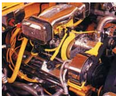
High thermal and chemical resistance and wide color/size selection make PET ideal for customizing and protecting the wires, hoses and cables in custom and classic cars.
