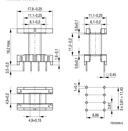
Hole arrangement View in mounting direction
