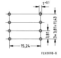
Hole arrangement View in mounting direction
