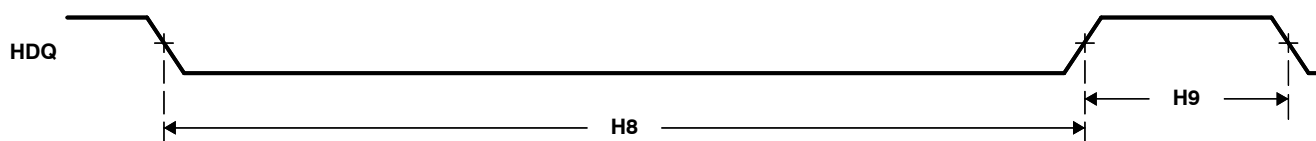
Figure 5–39. HDQ/1-Wire Break (Reset) Timing
