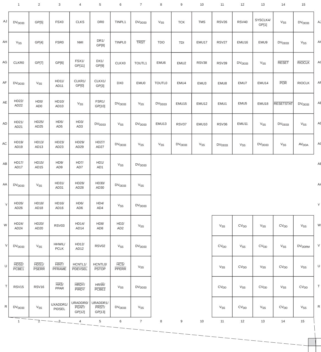
Figure 2-2. C6455 Pin Map (Bottom View) [Quadrant A]
