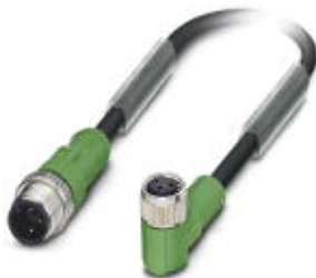
Sensor/Actuator cable, 3-position, PUR halogen-free, Black-gray RAL 7021, Plug straight M12, A-coded, on Socket angled M8, Cable length: 0.6 m
