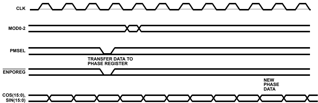
FIGURE 9. PHASE MODULATION TO OUTPUT DELAY
