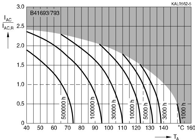
**Useful life<sup>1)</sup>**depending on case temperature  $T_C$  under ripple current operating conditions at  $V_R$
