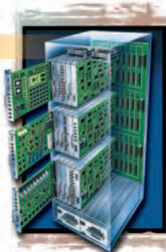
Carrier Rack Equipment
