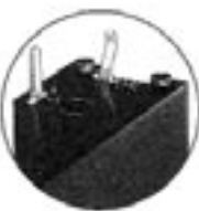
CLOSE-UP OF "Snap-In" TERMINAL
