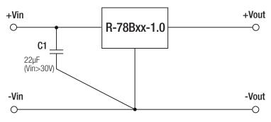
To protect the converter during power-up, use  $C1=22\mu F$  if Vin>30V
