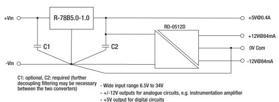
Isolated, wide Input range, Distributed Power Architecture (Point of Load)
