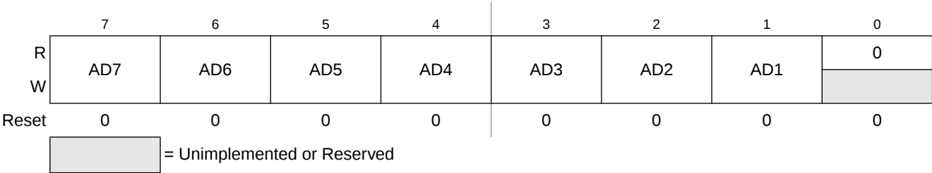
Figure 11-3. IIC Address Register (IICxA)
