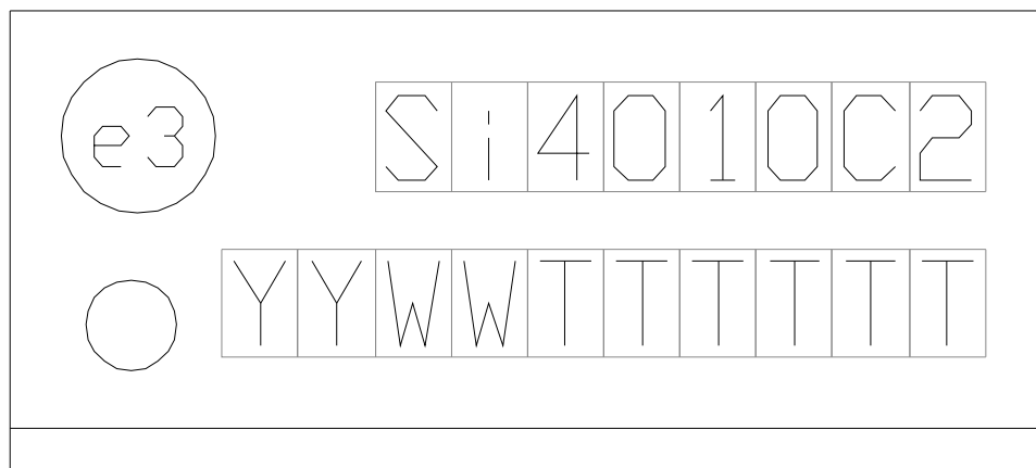
Figure 1. Si4010 Top Marking
