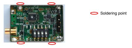
For stable module operation, It is recommended to solder the shield case to PCB wide GND (see above)
