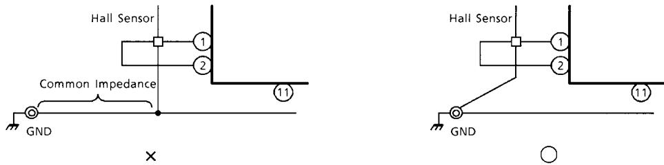
To decrease noise problems, we recommend to connect noise suppression capacitance (0.001 to 0.02  $\mu$ F) between each Hall Input Terminal.
