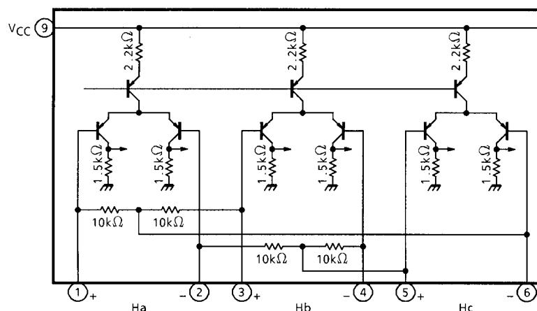
Wide DC operating range of 0 to  $V_{CC} - 1.2$  V is accomplished by PNP input circuit and also built in hysteresis restricts mis-function caused by external noise.
