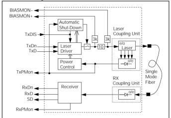
The receiver component converts the optical serial data into PECL compatible electrical data (RxD and RxDn). The Signal Detect (SD, active high) shows whether an optical signal is present<sup>(1)</sup>. If no optical input signal is present the receiver data outputs are switched to static low level (RxD=0, RxDn=high).
