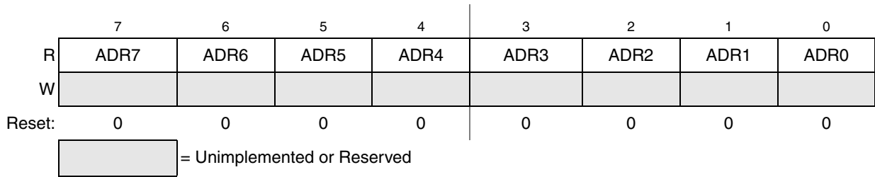
Figure 9-7. Data Result Low Register (ADCRL)
