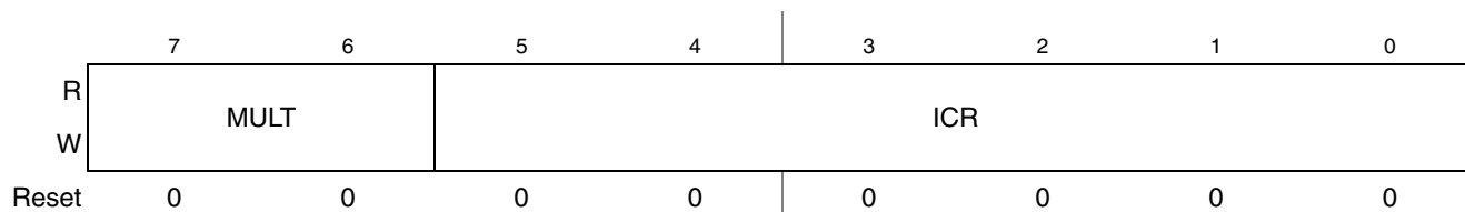
Figure 11-4. IIC Frequency Divider Register (IICF)
