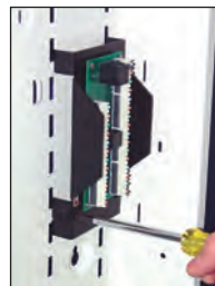
Step 2 - Secure with two screws
