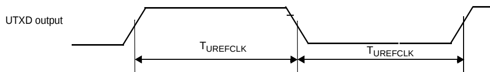
Figure 22. UART Output Timing
