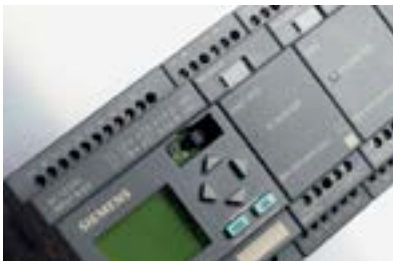
LOGO! in assemblies with the function modules
