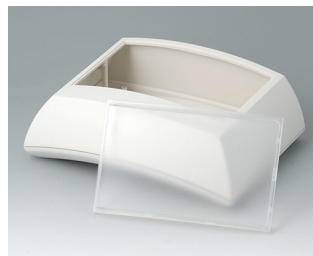
B7025247 ERGO-CASE L, high ABS (UL 94 HB) off-white RAL 9002 5.91"x7.87"x2.72" IP 40
