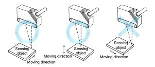
Install the Sensor as shown in the following illustration if each sensing object greatly differs in color or material.
