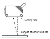
If the sensing object has a glossy surface, however, incline the Sensor by  $5^{\circ}$  to  $10^{\circ}$  as shown in the illustration, provided that the Sensor is not influenced by background objects.
