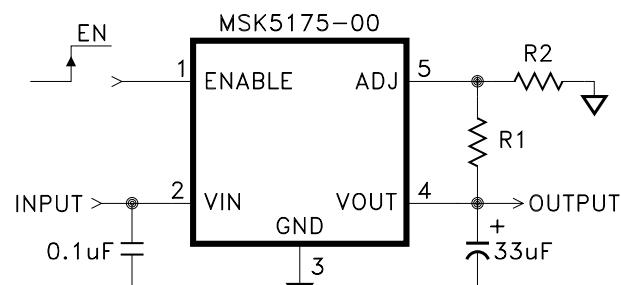
$$V_{OUT} = 1.240V \times [1 + (R_1/R_2)]$$
