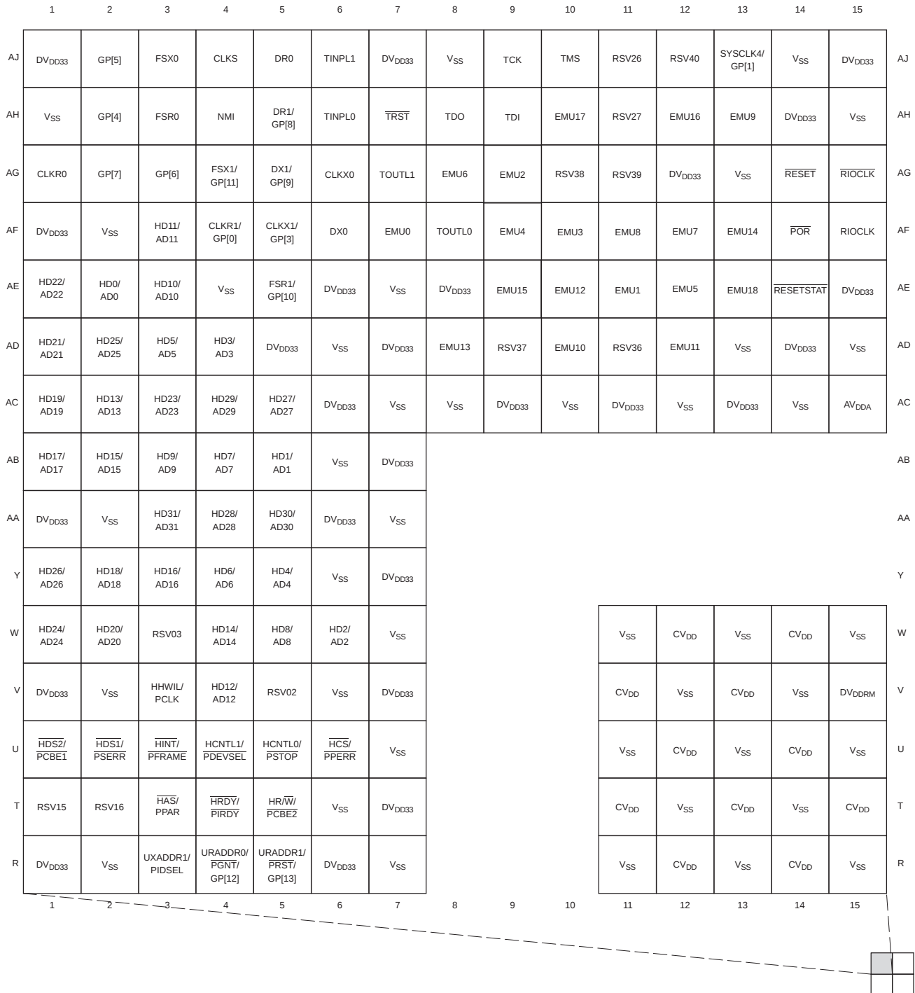
Figure 2-2. C6455 Pin Map (Bottom View) [Quadrant A]
