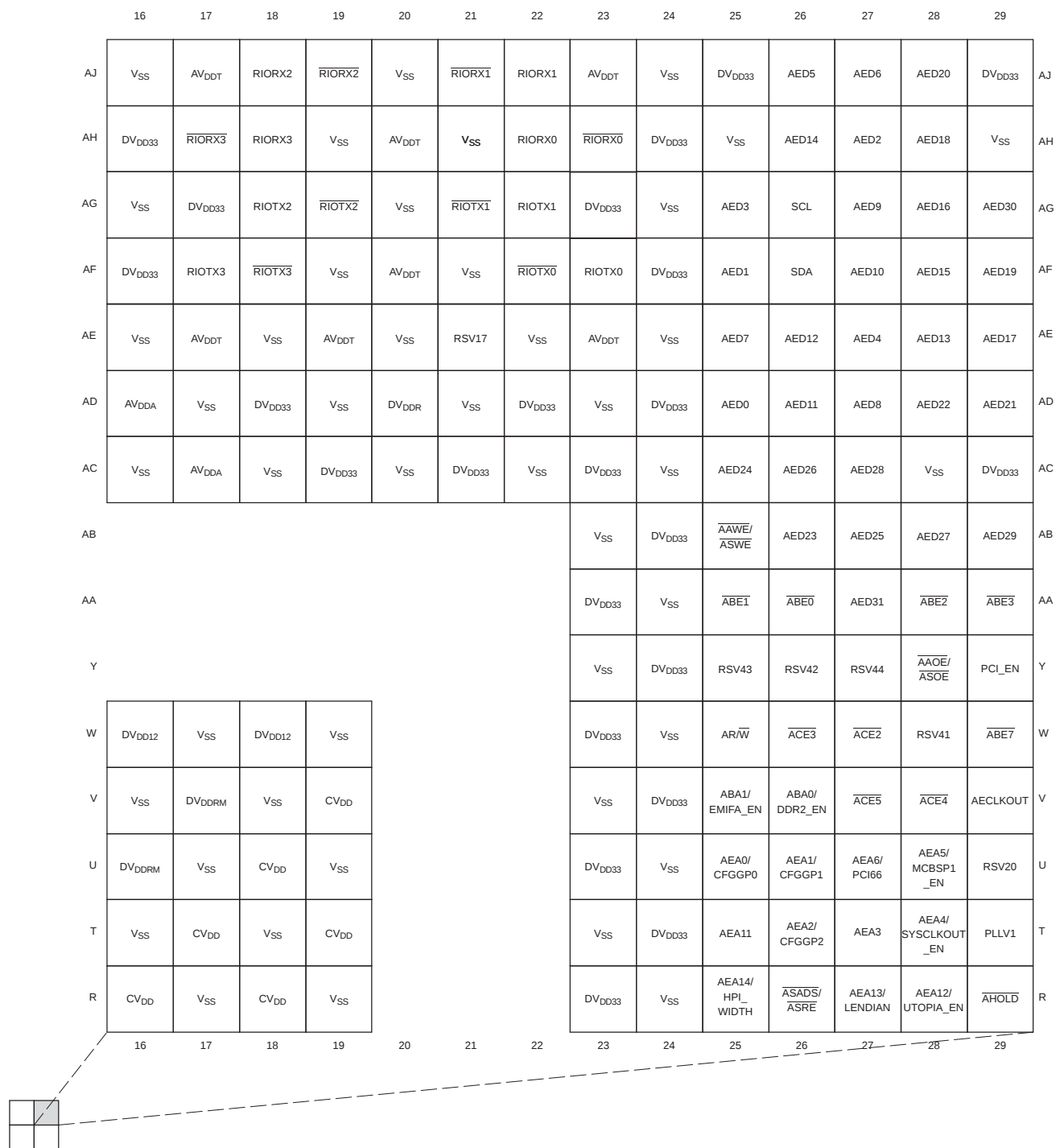
Figure 2-3. C6455 Pin Map (Bottom View) [Quadrant B]
