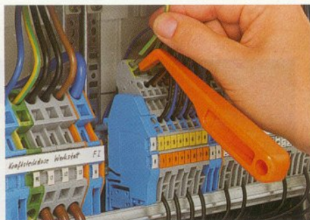
Operation of topJob terminal blocks for wire sizes from 2.5 mm 2 – 16 mm 2 /AWG 14 – 6, ideal with the universal topJob tool.
