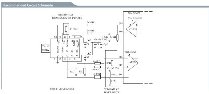
The split-load terminations for ECL signals need to be located at the input of devices receiving those ECL signals. The power supply filtering is required for good EMI performance. Use short tracks from the inductor L1/L2 to the module  $R_X V_{CC}$  and  $T_X V_{CC}$ . A GND plane under the module is required for good EMI and sensitivity performance.
