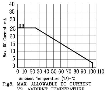
Fig8. MAX. ALLOWABLE DC CURRENT
