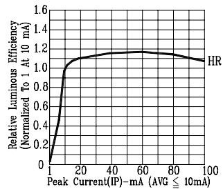
Fig4. RELATIVE LUMINOUS EFFICIENCY
