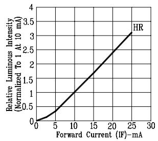
Fig3. RELATIVE LUMINOUS INTENSITY
