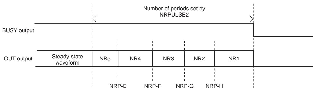
The fall waveforms are output in order from the NR5 waveform to the NR1 waveform. The switching timing is set in the same manner as that for rise operation.
