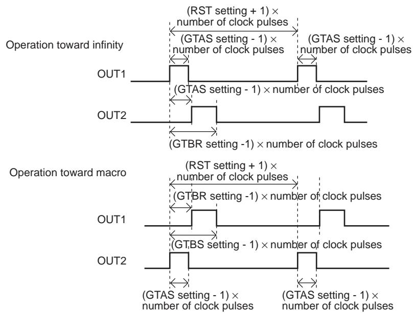
Sequence of initial setting operation (“on” or “off” can be set by the serial settings.)
