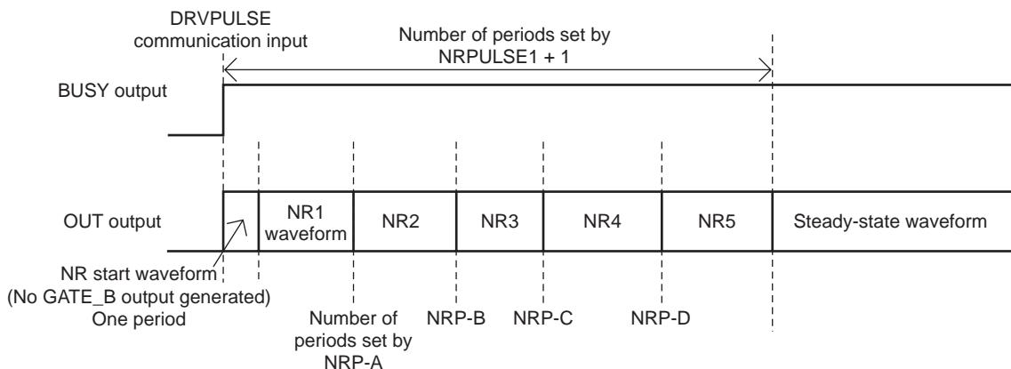
For example, when NRPULSE1 is set to 15, NRP-A to 3, NRP-B to 6, NRP-C to 9, and NRP-D to 12, one period of the NR start waveform (no GATE\_B output) is output, followed by three periods of the NR1 waveform, three periods of the NR2 waveform, three periods of the NR3 waveform, three periods of the NR4 waveform, three periods of the NR5 waveform, and then  $STP \times DRVPULSE$  periods of the steady-state waveform.
