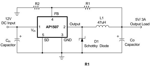
$$V_{OUT} = V_{FB} \times (1 + \frac{R1}{R2})$$
