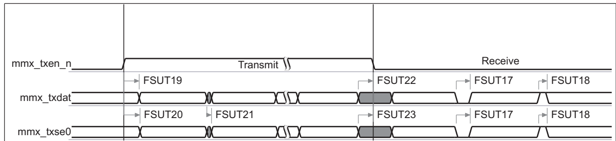
Figure 6-48. Low-/Full-Speed USB – Bidirectional TLL 3-pin Mode
