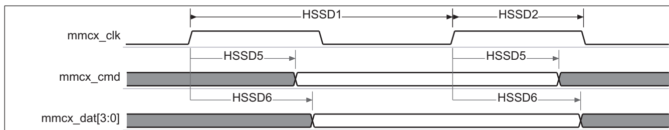
Figure 6-65. MMC/SD/SDIO – High-Speed SD Mode – Data/Command Receive
