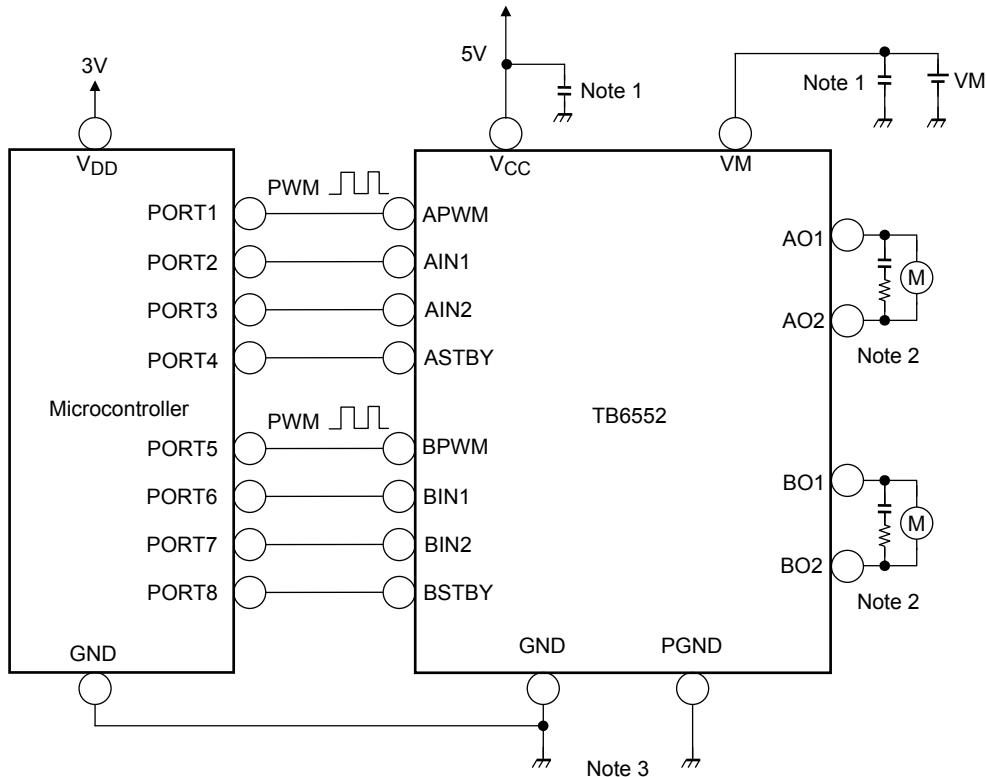
Note 1: The power supply capacitor should be connected as close as possible to the IC.
